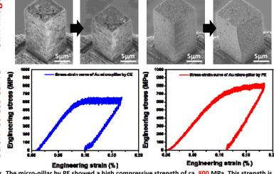
PE favors the nucleation of Au nuclei and greatly increase the Au nuclei density . The micro-pillar by PE showed a high compressive strength of ca. 800 MPa. This strength is much higher than ca. 600 MPa of the micro-pillar fabricated from Au film fabricated by CE.
